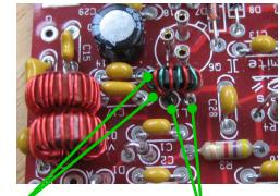
Connect secondary leads, to two S pads at ends of C14 and C17 pads
